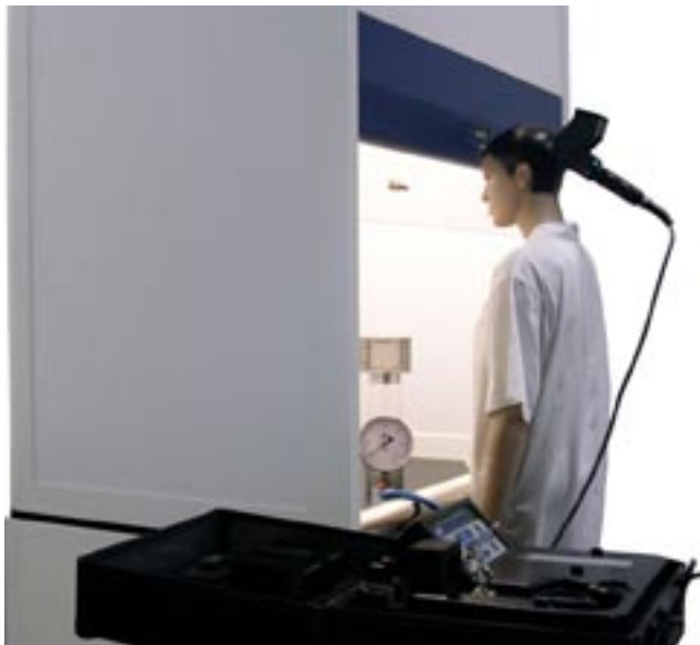
1. Tracer gas containment test
